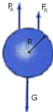
FIGURE 2.5 – Sédimentation : illustration
